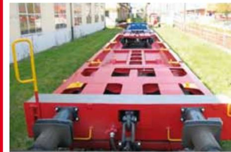
transit, in collaboration with the Ticino rolling stock manufacturer, Ferriere Cattaneo. Derived from the MEGA wagon, it features an increased load capacity and greater mileage. Environmental performance has also been improved: a combined synthetic pad and disc brake makes for lower noise levels. Testing of the prototype will run until the end of 2012.
