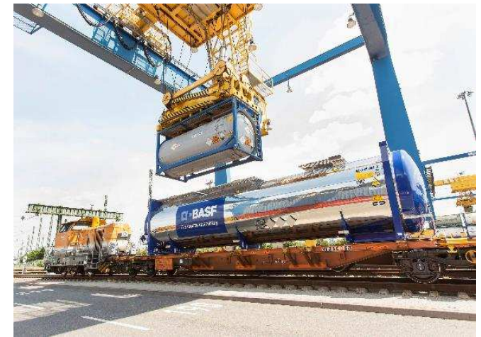
Standard tank container 25,000-36,000 liter volume 25 tons payload
